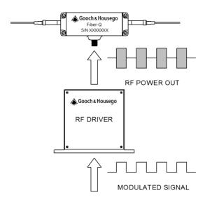
To use a fiber coupled acousto-optic modulator (AOM), connect the two fiber ports (reciprocal) into the light path, then connect the driver to the AOM SMA connector using a suitable RF cable.
