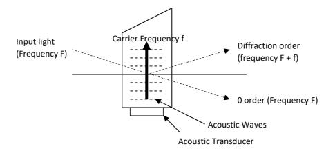
A radio frequency (RF) signal applied to the piezoelectric transducer generates a travelling acoustic wave in the bulk material. This acoustic wave produces a refractive index 'grating'. Incident light is diffracted from this grating.
